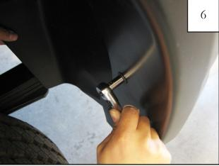
Holding flare in position on fender, reinstall screws removed in Step 5. Do not tighten at this time. *Note:* An Awl may be used to align the threaded clip with holes in flare and fender lip. Make sure screws engage in splash sheild.
